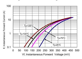
Figure 3: Typical Forward Voltage
