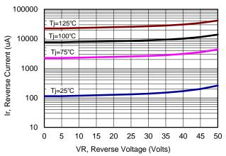
**Figure 4: Typical Reverse Current**
