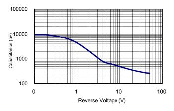
**Figure 5: Typical Junction Capacitance**
