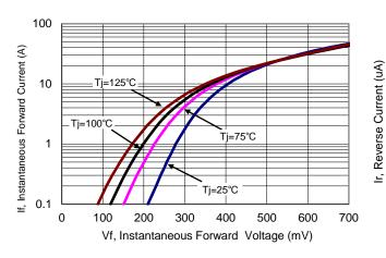
Figure 3: Typical Forward Voltage
