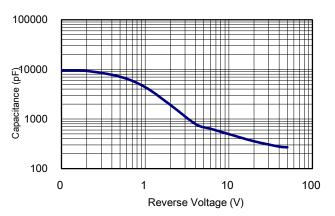
Figure 5: Typical Junction Capacitance
