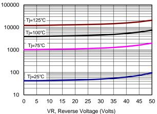
Figure 4: Typical Reverse Current
