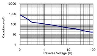
**Figure 5: Typical Junction Capacitance**
