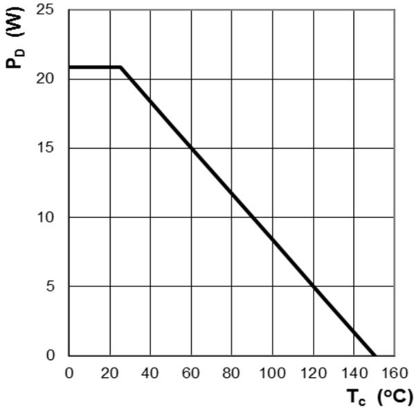
Figure 1: Power Dissipation
