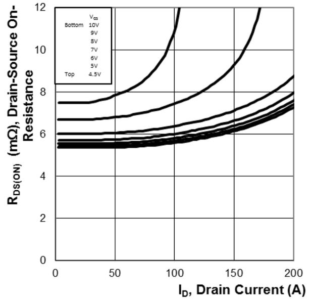
Figure 6: Typ.  $R_{DS}$  Variation vs.  $I_D$  and  $V_{GS}$
