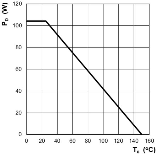
Figure 1: Power Dissipation
